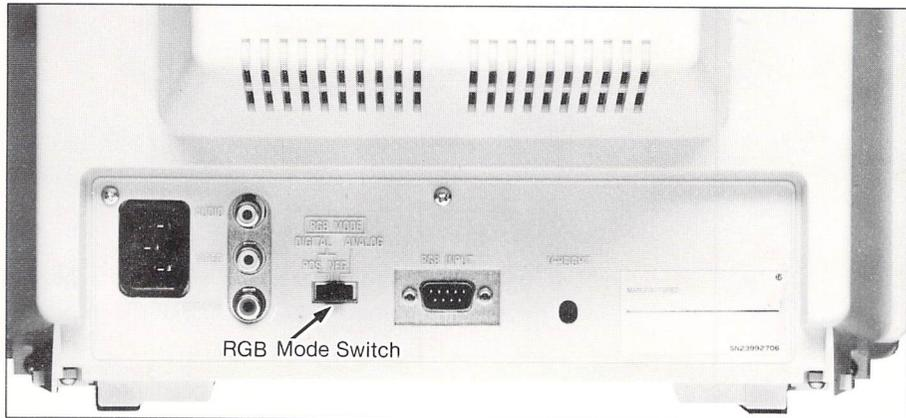
2. Set the RGB MODE SWITCH (on the back of the monitor directly to the left of the RGB INPUT socket) to Analog display mode. The switch should be set to the far right.
