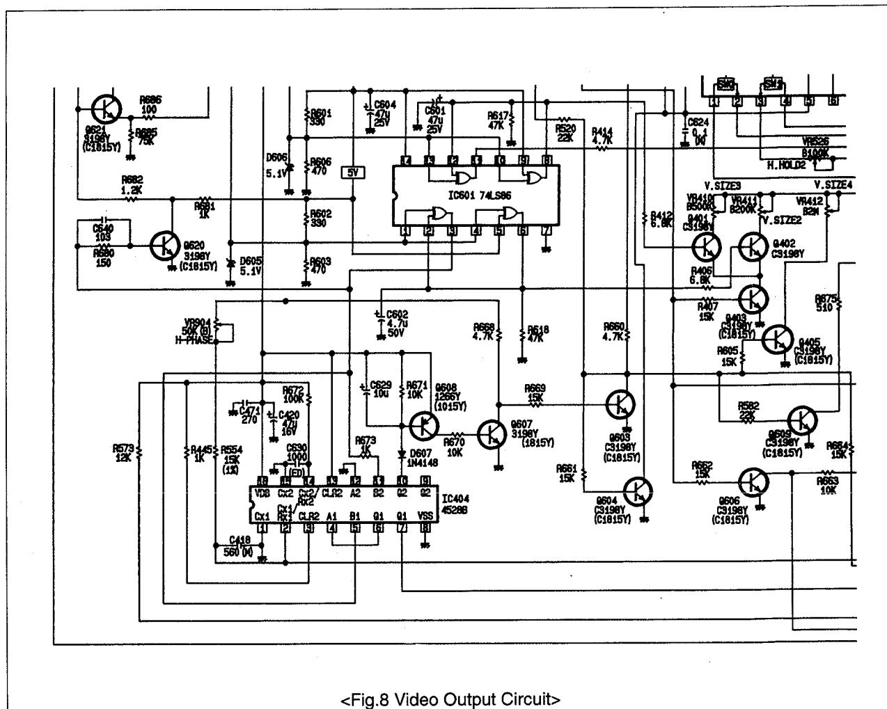
Vertical size and linearity of VGA mode are determined by the horizontal and vertical sync polarity using exclusive or gate IC (IC601 74LS86). The polarity of each IC 601 pin is as follow:
