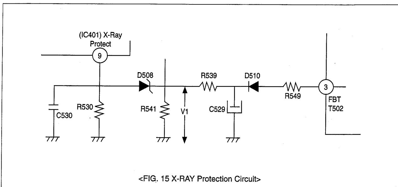
The Pin 3 Winding of the flyback transformer supplies current to the protection circuit. D510 rectifies the current before it is applied to the R539. This DC current is divided by R539 and R541. Incase of normal operation, the voltage V1 is lower than the D508's breakdown voltage. When the high voltage exceeds specifications by about 20%, voltage V1 exceeds D508's breakdown voltage.
