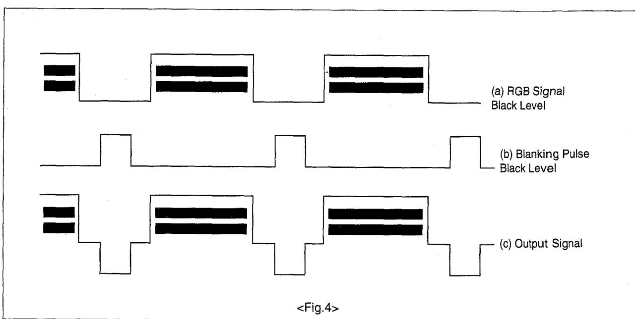
This amplitude of blanking pulse can be adjusted by voltage applied to terminal 20 of TA8631N.
