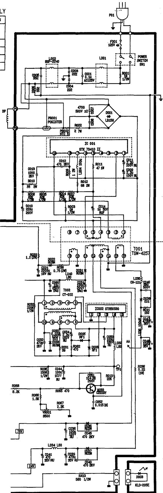
The voltage is regulated controlling the positive bias of TR1.
