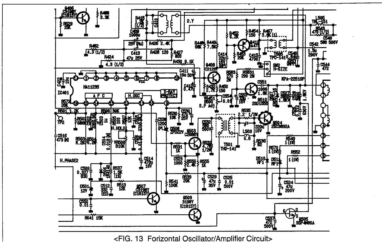
Horizontal synchronizing signal is input into IC401 through pin 15.
