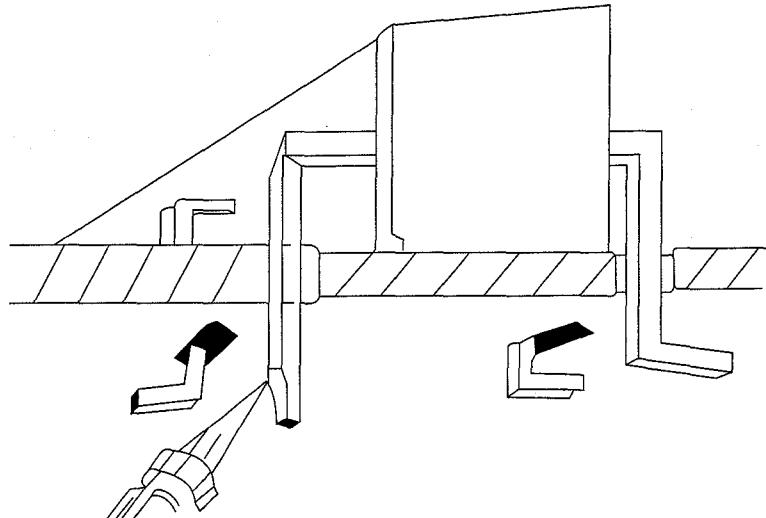
FIGURE 1. USE SOLDERING IRON TO PRY LEADS
