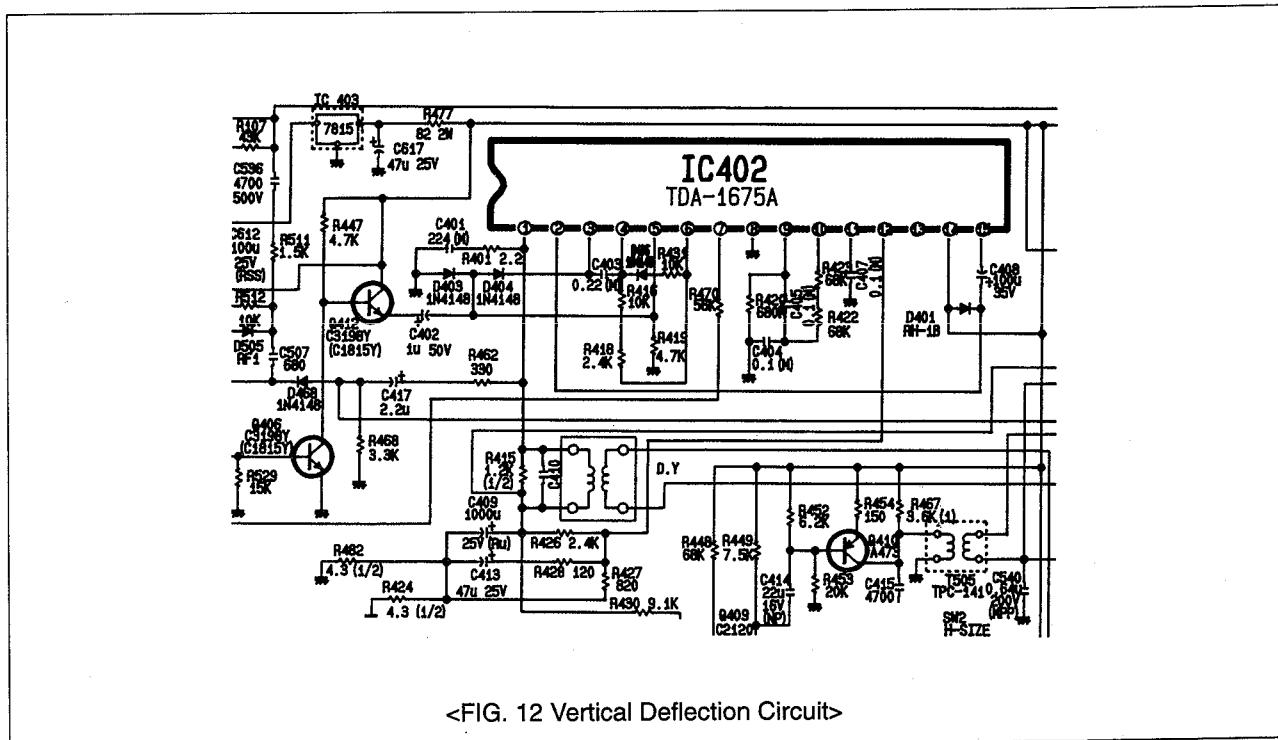
Q406 inverts the vertical sync pulse to develop a positive-going pulse at its collector.
