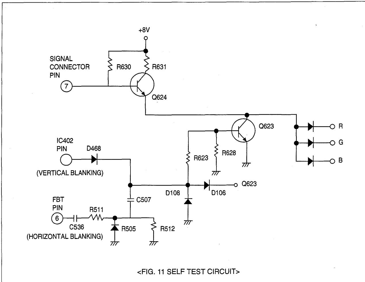
Self-test pattern should be available when the contrast control is rotated its maximum. With the signal cable disconnected, the display shows full white raster which should extends beyond the bezel at the top and bottom. The brightness should be uniform in the region extending from the screen center. With the brightness control detent, the brightness of the raster should be greater than 10 Ft-L.
