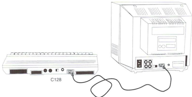
BE SURE TO DISCONNECT THE POWER TO BOTH THE MONITOR AND THE COMPUTER TO PREVENT DAMAGE BY SHORTING.
