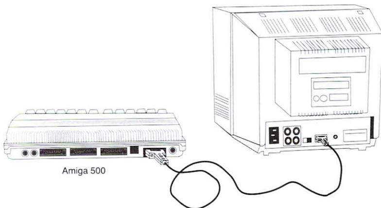
First, TURN OFF THE POWER TO BOTH THE MONITOR AND THE COMPUTER TO PREVENT DAMAGE BY SHORTING. Next, connect the video cable. Simply insert the small, rectangular 9-pin D connector into the port labeled **RGB Input** on the back of your 1084. Then insert the other end of the cable with the large, 23-pin RGB connector into the video port on the back of your Amiga. Tighten the screws that are on each side of the connectors.
